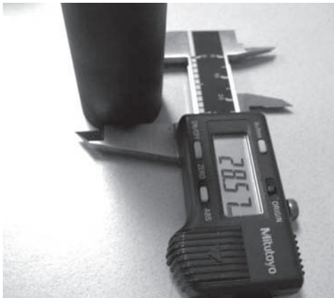
Checking steerer tube size
