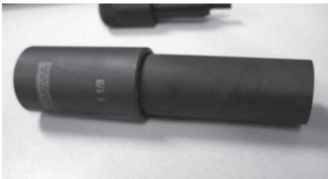
Using steerer tube section as gauge
